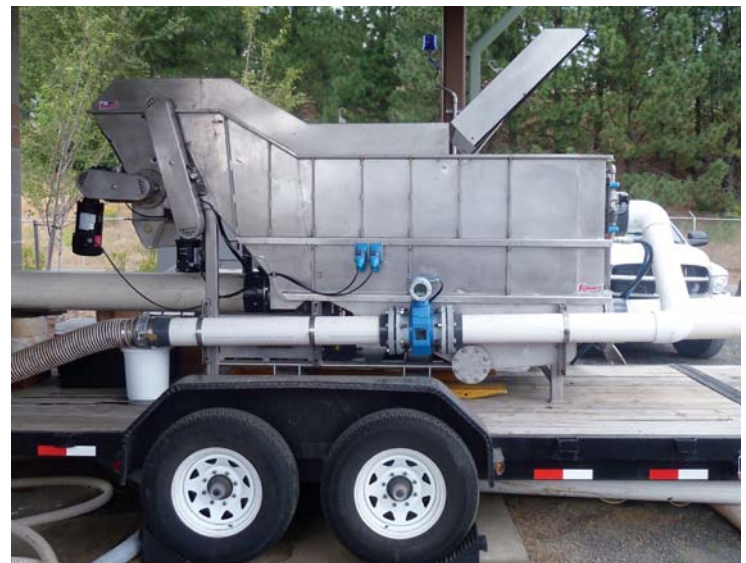
Figure 3. 1.7 mgd Capable Unit Tested at Plummer Wastewater Treatment Plant
